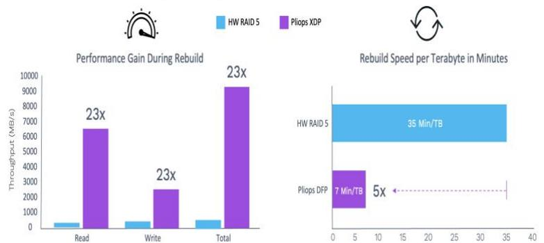
Figure 3: XDP Performance During Rebuild and Rebuild Speed
