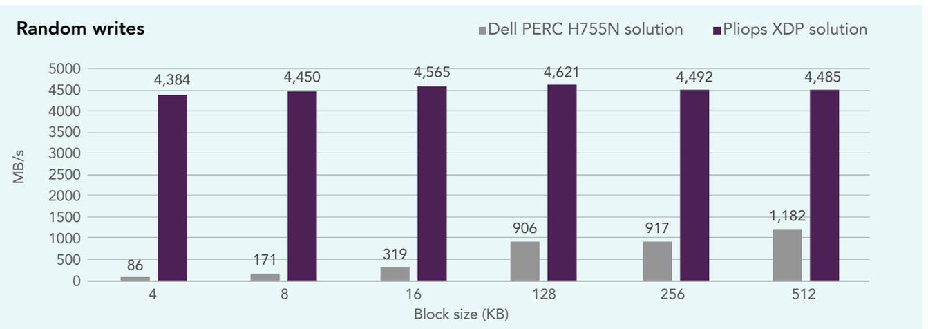
Figure 2: Random write bandwidth, in MB/s, at multiple block sizes for the Pliops XDP and Dell PERC H755N front NVMe solutions. Higher numbers are better. Source: Principled Technologies.
