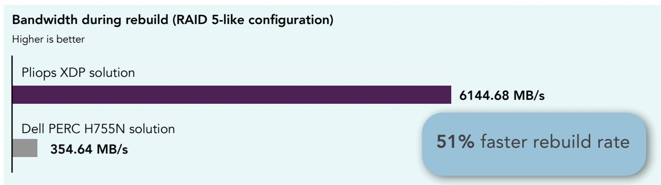
Figure 3: Bandwidth, in MB/s, during a drive rebuild (four-drive RAID 5 array with high-priority rebuild settings). Higher numbers are better. Source: Principled Technologies.
