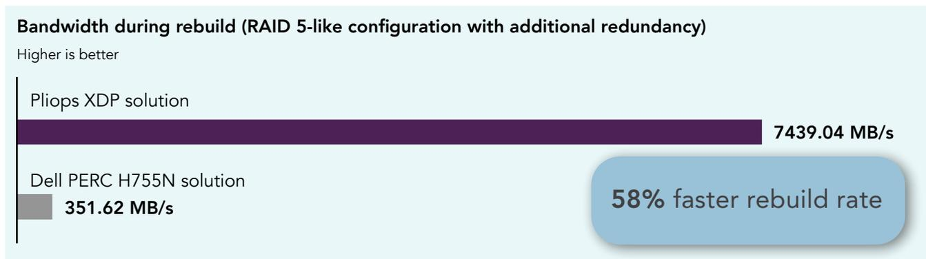
Figure 4: Bandwidth, in MB/s, during a drive rebuild (RAID 5 array with additional redundancy with high-priority rebuild settings). Higher numbers are better. Source: Principled Technologies.
