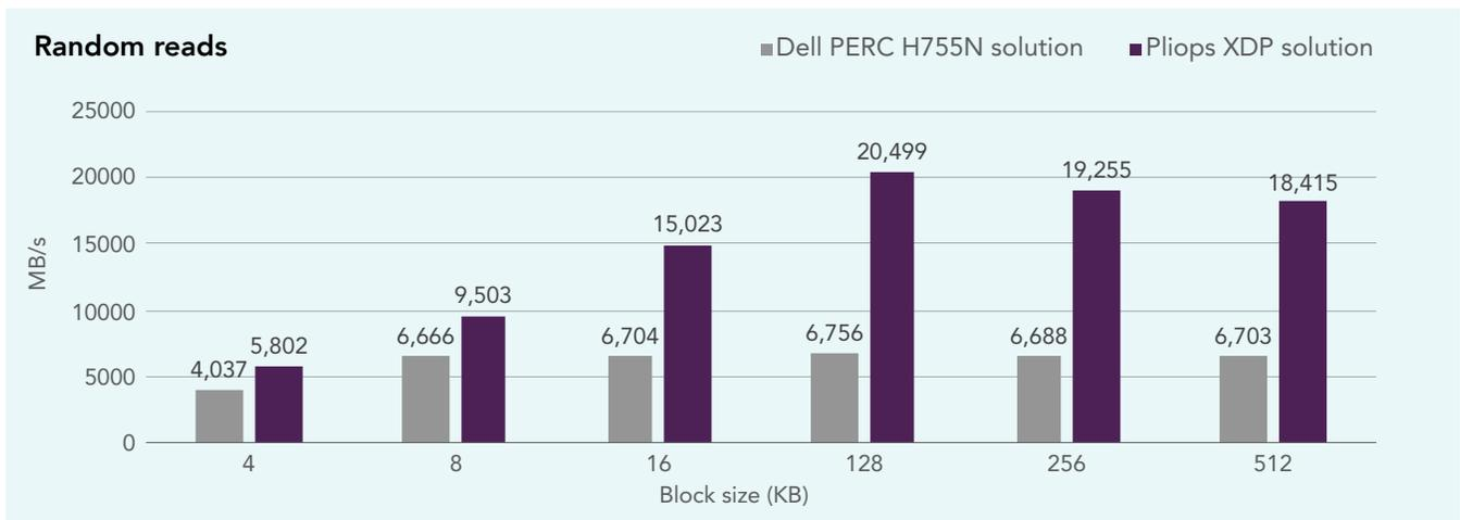
Figure 1: Random read bandwidth, in MB/s, at multiple block sizes for the Pliops XDP and Dell PERC H755N front NVMe solutions. Higher numbers are better. Source: Principled Technologies.
